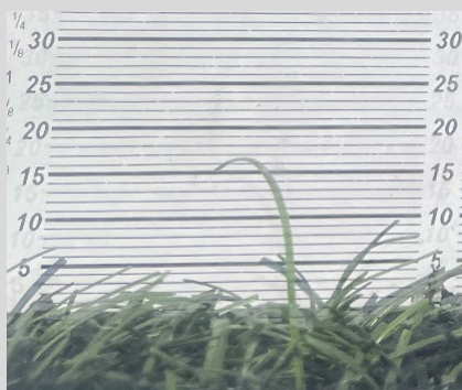
Figure 5 - Free pile height in Location 2 (far side penalty)
